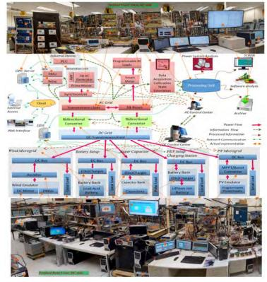
The FIU Smart Grid Testbed is located at the facility of the Energy Systems Research Laboratory in the Department of Electrical Engineering, College of Engineering and Computing at Florida International University in Miami, Florida. It is a state of the art hardware -software platform for research and development, component evaluation, as well as educational activities.
